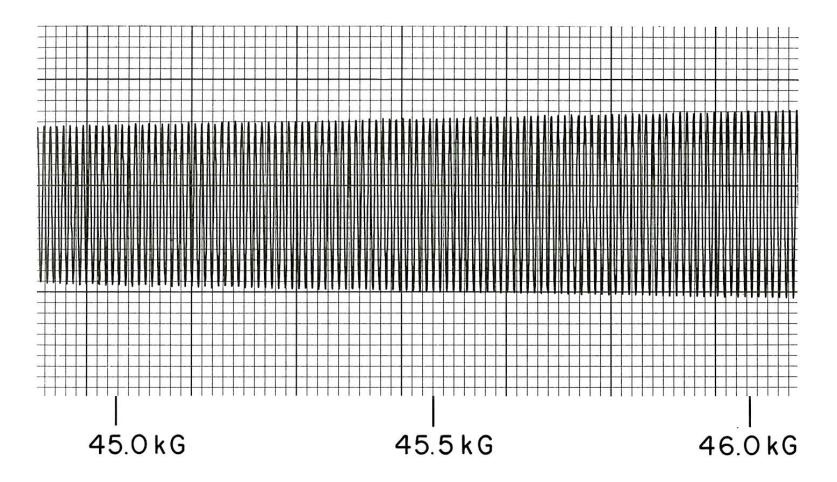
Figure 31 De Haas-van Alphen effect in gold with  $\mathbf{B} \parallel [110]$ . The oscillation is from the dog's bone orbit of Fig. 30. The signal is related to the second derivative of the magnetic moment with respect to field. The results were obtained by a field modulation technique in a high-homogeneity superconducting solenoid at about 1.2 K. (Courtesy of I. M. Templeton.)
