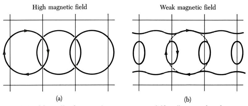
Figure 33 Breakdown of band structure by a strong magnetic field. Brillouin zone boundaries are the light lines. The free electron orbits (a) in a strong field change connectivity in a weak field (b) to become open orbits in the first band and electron orbits in the second band. Both bands are mapped together.
