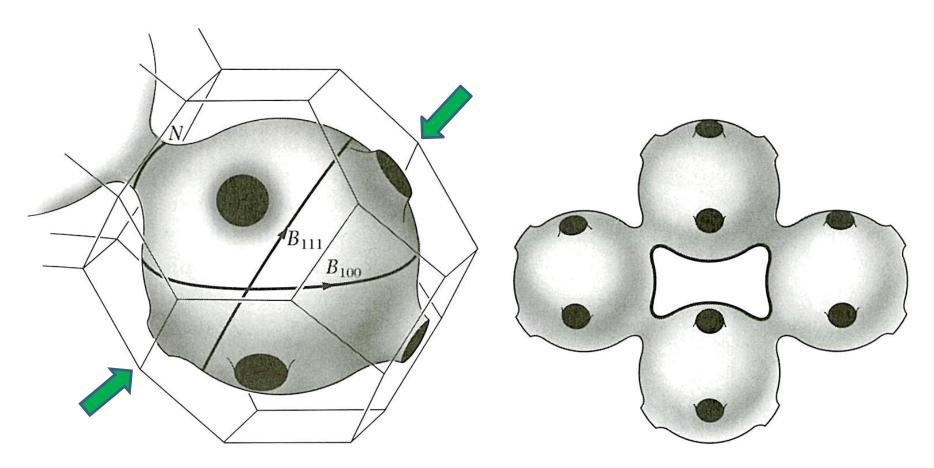
Figure 29 Fermi surface of copper, after Pippard. The Brillouin zone of the fcc structure is the truncated octahedron derived in Chapter 2. The Fermi surface makes contact with the boundary at the center of the hexagonal faces of the zone, in the [111] directions in **k** space. Two "belly" extremal orbits are shown, denoted by *B*; the extremal "neck" orbit is denoted by *N*.
